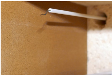
Typical installation of a thermocouple inside an oven. Two blank wires go through a ceramic tube with two holes. Ends are drilled together.
