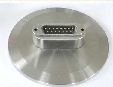
Sub-D thermocouple feedthrough 15 pins (7 pairs) on a KF50 flange. Upper row are the (+) pins, lower row the (-) pins. Pins are not plated.
