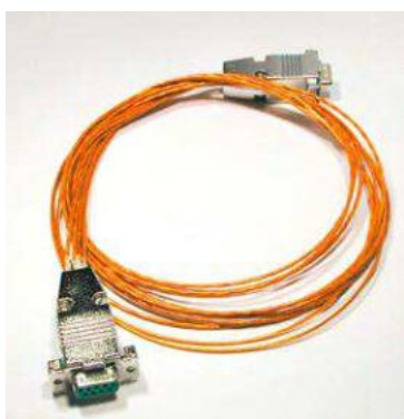
Example of two custom cables: Top: Single wires used with HV Sub-D connectors including housing and strain relief
