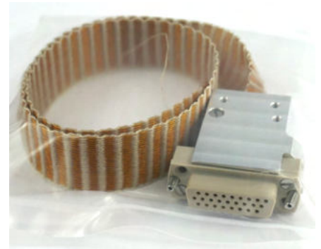
Top: 26 pin HD connector with housing and 26way ribbon cable
