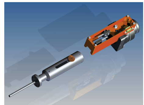
Micro-switches and motor removed for bakeout.
