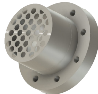
The Ultra Low Pressure Burst Disc with a rupture pressure below 0.5 bar on 63CF flange. With this component, the overpressure regulations do not apply for the system. Mesh Cover to prevent accidental damage to the membrane
