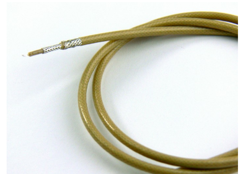
Double shielded PEEK Triaxial cable, 50 Ohm Impedance, 310-PEEK50-TRIAX
