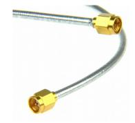
380-SMA18G-MM-300: Ready made RF cable for UHV use. As PTFE must be used for high frequency cables, the cable is not radiation resistant
